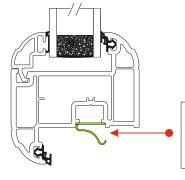
Fit a **BC002** Sash Spring to the sash on the center line of the stay fixing
